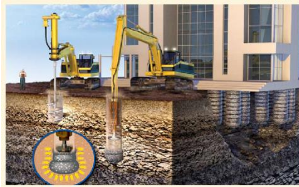
Figure 29: Example of RAP installation
