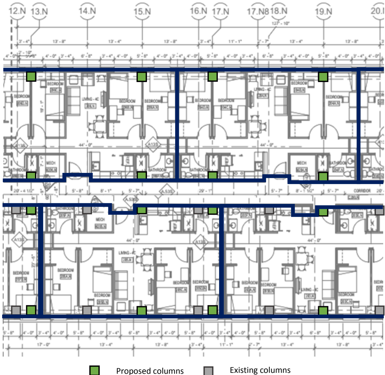
Figure 23: Apartment layouts with shifted columns
